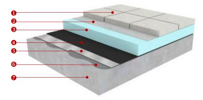
The Elevate Inverted System is a variation of the conventional ballasted system. It is ideal for roofs with regular traffic, or roofs in severe weather climates. It can be applied on any building that can accommodate the extra load of the ballast and where the roof slope does not exceed 10%.
