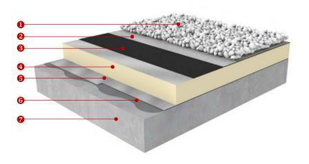
Elevate's EPDM Ballasted System is an economical EPDM roofing system, suitable for a wide variety of buildings. It can be applied on any building that can accommodate the extra load of the ballast and where the roof slope does not exceed 10%.
